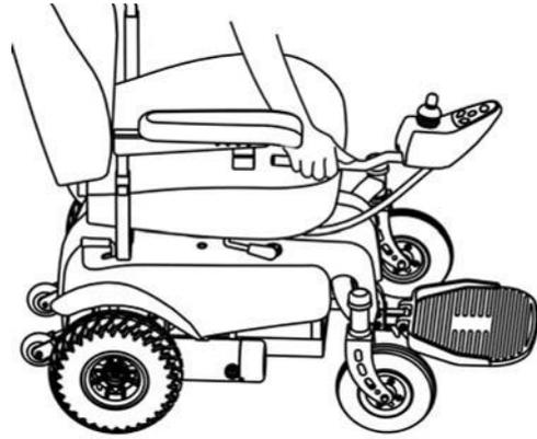
5. Pull the swivel lever up to unlock it and rotate the seat to the position where you can pull the seat up.
