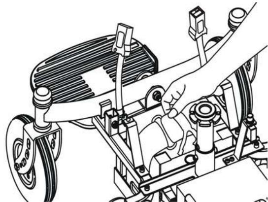
3. From the main cable, there are five connectors. Two connectors are for batteries; two connectors are for the motors and one to the controller.
