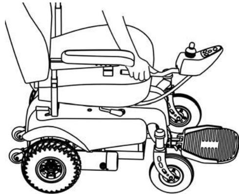
10. Rotate the knob to secure the controller.
