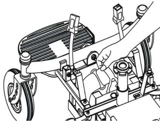
11. Remove the batteries.
