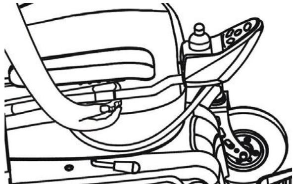
11. Press the power button. The battery gauge will turn on. The power system is now standing by.
