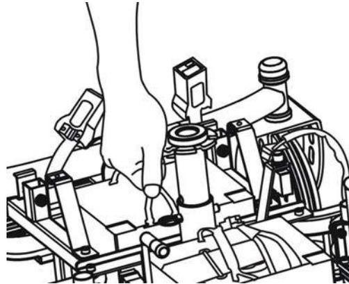
2. Fasten batteries with safety straps.
