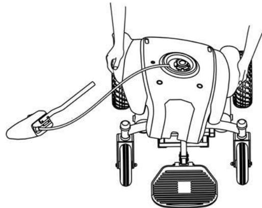
7. Lift the seat and pull the swivel lever up at the same time. Slide the bottom of the seat into the seat pedestal.
