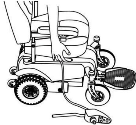
9. Take the controller (round tube) and insert it into the tube under the armrest.
