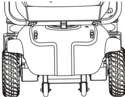
3. Rotate the knob to loosen the tube of the controller.
