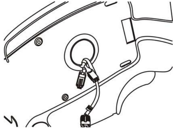
5. Connect both motor connectors with the main cable. Left connector to Left one, right connector to right one. (Left/Right indications are labeled on the wires).
