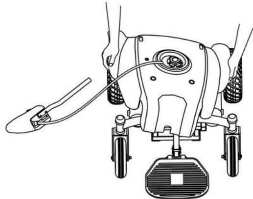
7. Disconnect the cable to the controller from the hole in the shroud.
