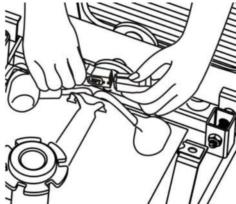
6. The shroud should also slide through the clutch levers—which should be positioned in engaged mode—and secure the shroud to the body frame. (Parallel to the wheels)
