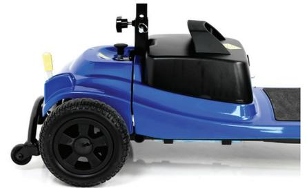
Battery box weighs only 3kg
