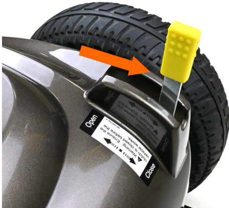
Fig 6.7.1 Drive Mode (Closed)
