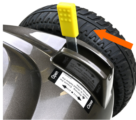
Fig 6.7.2 Freewheel Mode (Open)
